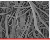
White PTFE fiber, shown in this magnified view, is inherently liquid repellant and resistant to harsh chemical attack. Its dense nature yields fine fiber sizes, further enhancing filtration performance.
